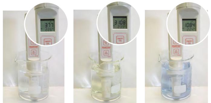
Check the Electrical Conductivity by means of a conductivity meter TESTER CST on mains water and water treated with Antinex+Thermakil® to 3 % and system water treated with Filmax+Thermakil® to 2 %.
