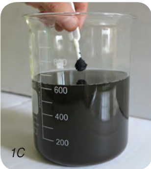
Fig 1A , 1B and 1C - Some examples of system water , respectively non-corrosive , corrosive and highly corrosive rich of magnetite
