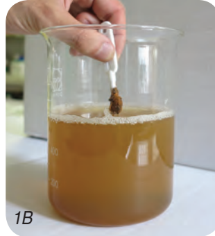
Fig 1A , 1B and 1C - Some examples of system water , respectively non-corrosive , corrosive and highly corrosive rich of magnetite
