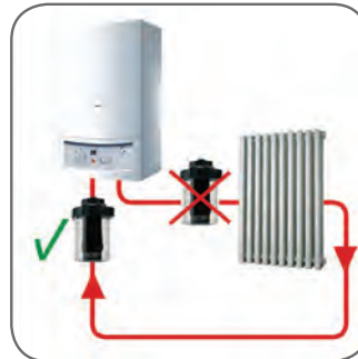
Figure 6 – MAG-NEX HP Proper Installation
