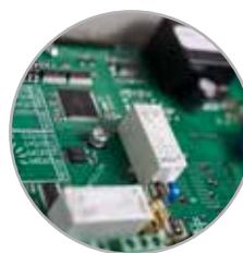
Trasformatori switching ad ampio range Wide range switching transformer
